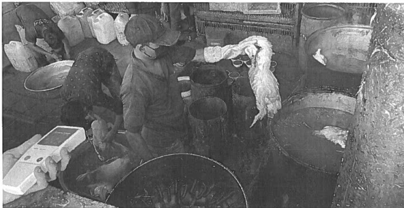
A handheld air sampler keeps watch for airborne viruses at a Cambodian market. The device can also be loaded onto a drone or toy car to reach inaccessible spots.
